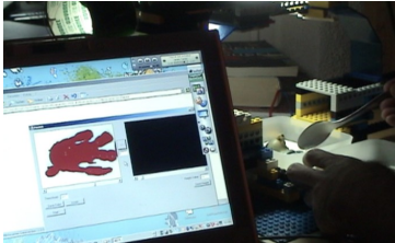
figure 2. A plastic robot in a tupperware bowl full of milk. On the left, we see the threshold image – all red pixels indicate the object, all the white pixels indicate milk.
