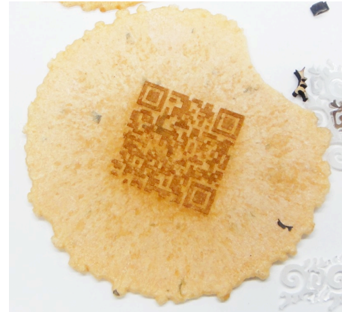
Figure 6. A 2D fiducial marker is embedded in a cracker.
