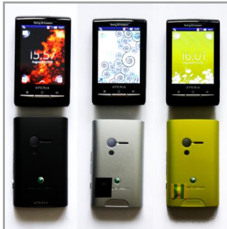
Figure 3. Mobile phone prototype using magnets on shells to control themes and other content.
