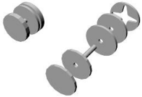
figure 16. The gear system for actuation of the flowers with servomotors
