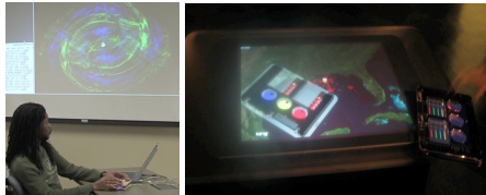
Figure 2 A. User uses physical dials to control a remote-generated visualization of black hole simulation data. B. Gulf of Mexico Oil Spill Data Visualization User Interaction can be driven by casier tangibles [15] that are mediated both by the MS Surface and Apple iPad.
