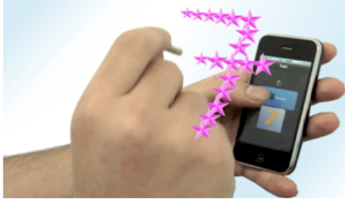
Figure 1. Entering text(digit) using the space around the device. The user simply draws the digits in the air using a properly shaped magnet taken in one hand.
