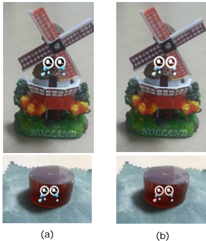
Figure 3: (a) Direct image blending and (b) Seamless image blending (Poisson image edit)
