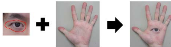
Figure 2: Poisson Image Edit blending example, its basic concept is gradient blending, not image itself, so it shows seamless blending result
