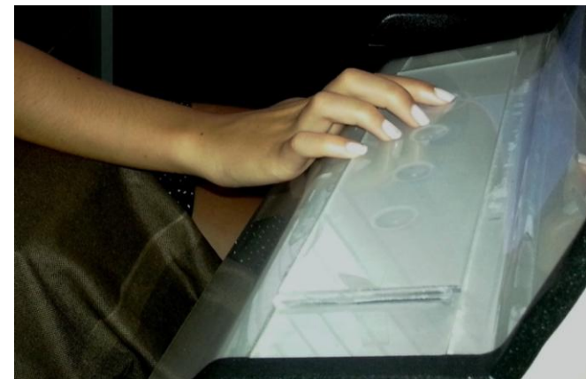
Figure 6. A user is performing a selection with DRAG_IN by positioning the hand on the convex bend, placing the fingers on the horizontally oriented surface and dragging into a hollow.
