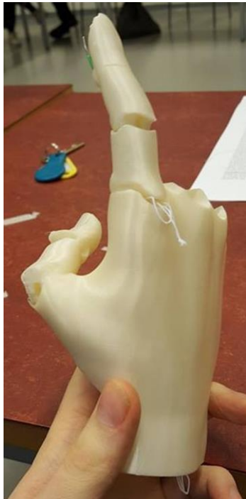
Figure 3: Functional fingers were acquired through elastic wiring inside the hand.
